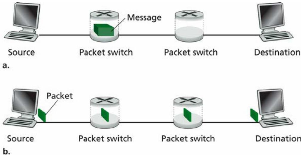
Figure: End-to-end message transport: (a) without message segmentation; (b) with message segmentation
