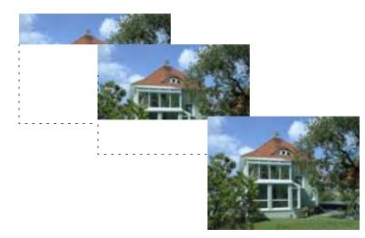
**Figure 7-15** Example of sequential picture preparation, here using the lossy DCT-based mode.
