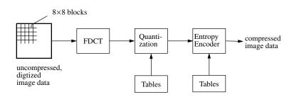
**Figure 7-9** Steps of the lossy sequential DCT-based coding mode, starting with an uncompressed image after image preparation.
