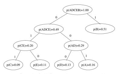
Figure 7-2 Example of a Huffman code represented as a binary tree.
