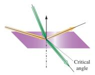
Figure 17.15 Total internal reflection.
