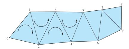
Figure 1.10 Triangle strip winding.
