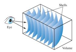
Figure 20.14 Slicing a 3D texture with spherical shells.
