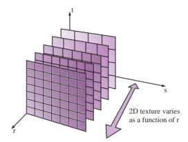
Figure 14.2 3D textures as 2D textures varying with R.
