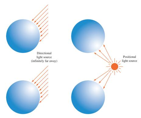
Figure 3.7 Directional and positional light sources.
