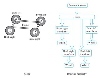
Figure 16.1 Instancing of four wheels.
