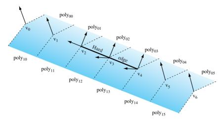
Figure 1.8 Splitting normals for hard edges.
