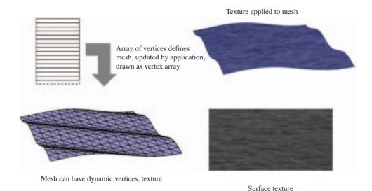
Figure 18.7 Dynamic mesh components.
