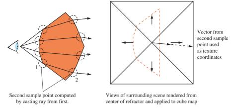
Figure 17.20 Refracting objects behind the refractor.
