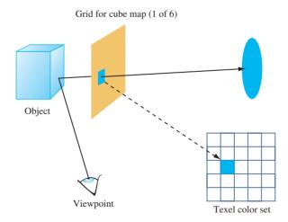
Figure 17.21 Creating environment maps using ray casting.
