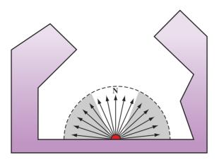
Figure 15.15 Cross section showing hemispherical visibility sampling.
