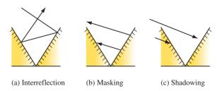
Figure 15.10 Interreflection, masking, and shadowing.
