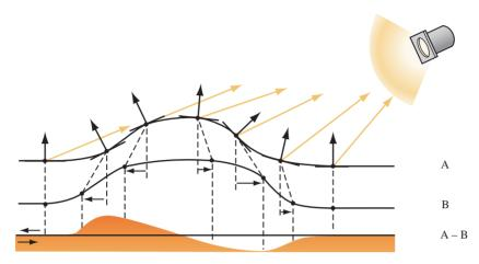
Figure 15.14 Shifting a bump map to perform forward differencing.
