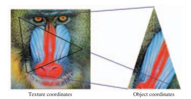
Figure 5.2 Vertices with texture coordinates. Texture coordinates determine how a texture maps to the triangle.
