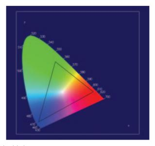
Figure 12.2 The CIE (1931) (x,y) chromaticity diagram.
