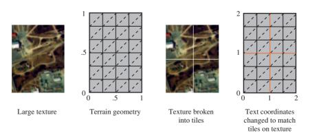
Figure 14.9 Modeling geometry to use texture wrapping.
