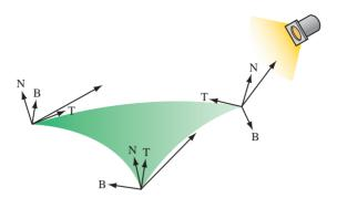
Figure 15.12 Tangent space defined at polygon vertices.
