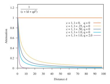
Figure 15.3 Attenuation function.
