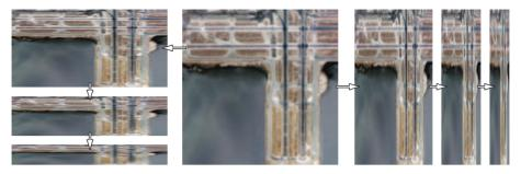
Figure 14.13 Creating a set of anisotropically filtered images.
