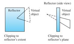
Figure 17.2 Clipping virtual objects to reflectors.
