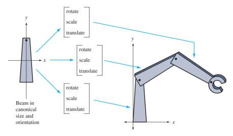
Figure 2.6 Modeling transform as part of model description.
