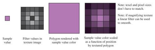
Figure 18.10 Using textures to filter a value.
