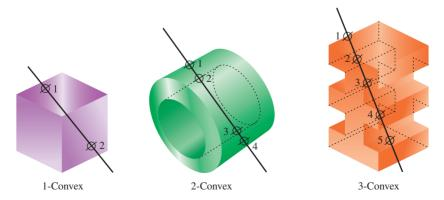
Figure 16.13 Examples of *n*-convex solids.
