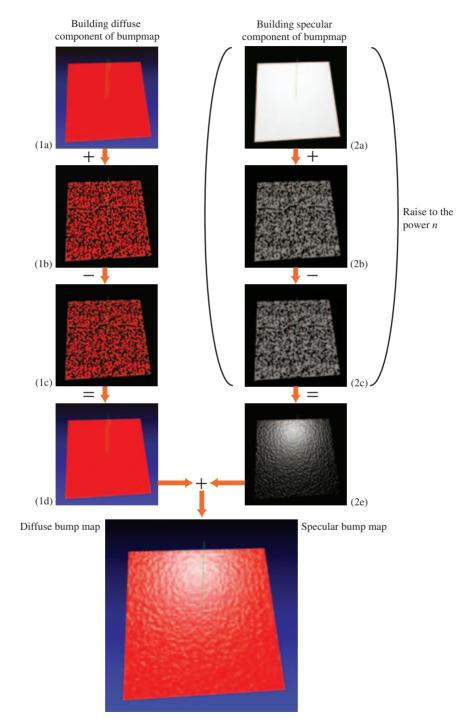
Figure 15.13 Bump mapping: shift and subtract image.
