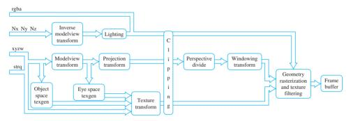
Figure 2.5 Texture coordinate transformation pipeline.
