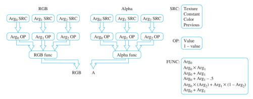
Figure 5.12 The components of the combine texture function.
