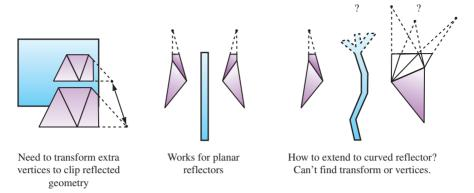
Figure 17.6 Clipping curved reflectors.
