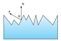
Figure 15.9 Surface modeled as a collection of V-cavities.
