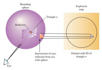
Figure 17.9 Mapping reflection vectors into explosion map coordinates.
