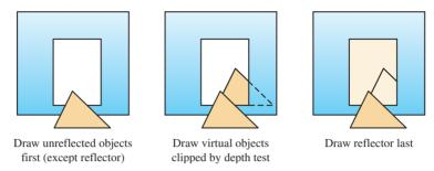
Figure 17.3 Masking reflections with depth buffering.
