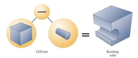
Figure 16.10 An example of constructive solid geometry.
