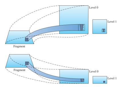
Figure 14.12 Pixel footprint on anisotropically scaled texture.
