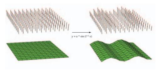
Figure 18.8 Water modeled as a height field.
