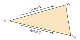
Figure 1.6 Computing a surface normal from edge cross-product.
