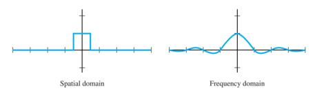
Figure 4.4 Box filter in spatial and frequency domain.
