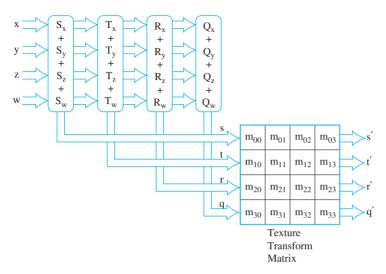
Figure 5.3 Linear texture coordinate generation.
