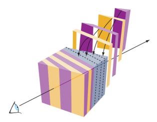
Figure 20.13 Slicing a 3D texture to render volume.
