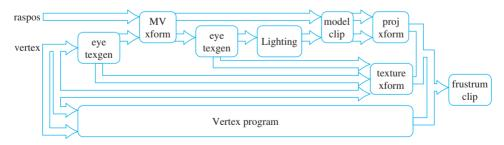
Figure 2.11 Vertex program and conventional transform modes.
