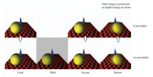
Figure 6.5 Accumulation buffer.
