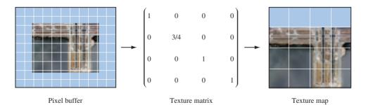
Figure 14.15 Non-power-of-two aspect ratio using texture matrix.
