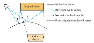
Figure 17.5 Normals and reflection vectors in curved reflectors.
