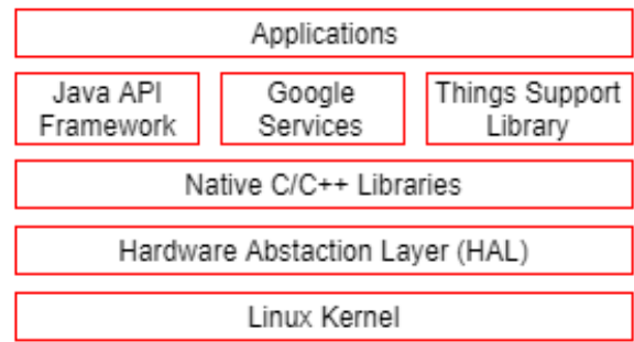
Fig. 2. Android Things architecture.
