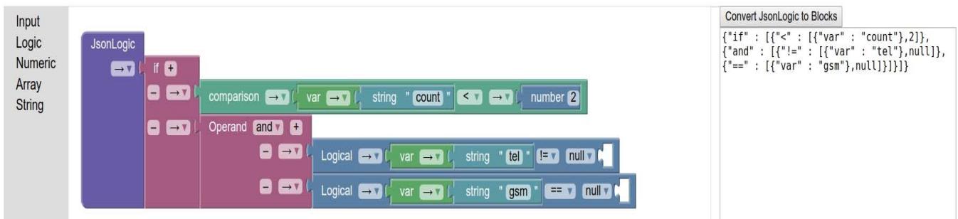
Fig. 3. Automatic update in the graphical models in case of any modification made inside JsonLogic textual structures
