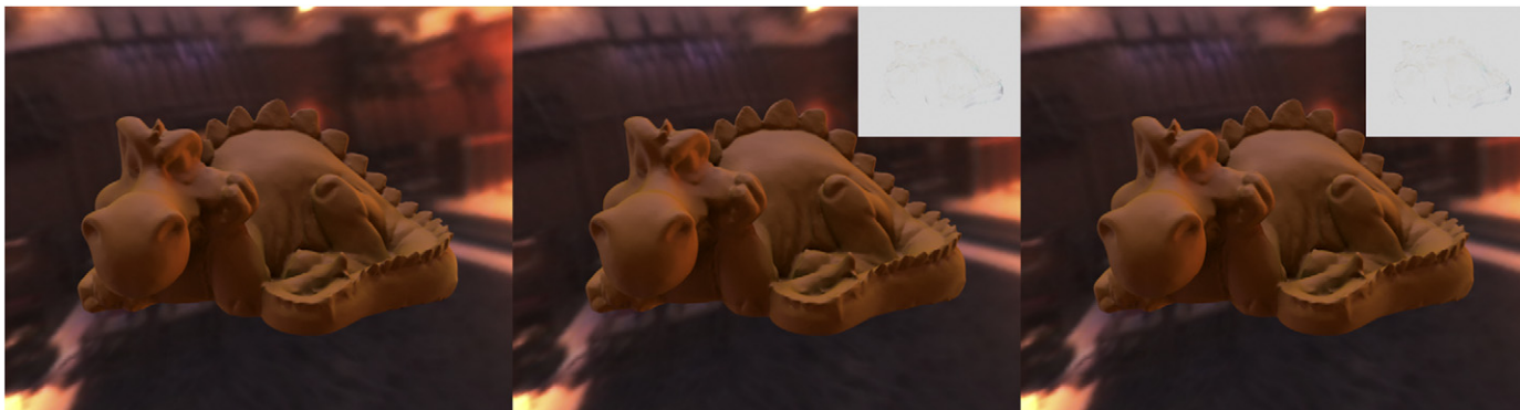
Fig. 8. Left: image based on the measured BRDF “orange-paint” [2]. Middle: scene rendered using polynomial model (Lafortune, p = 5 ). Right: scene rendered using the same polynomial model (Lafortune, p = 5 ) with incoming and outgoing light directions exchanged. Insets show a difference between the reference and the rendered images.
