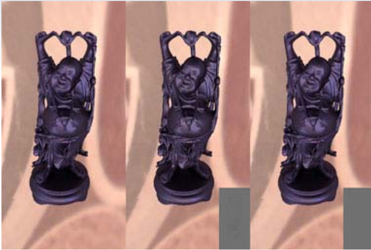
Fig. 1 - Monte Carlo renderings of a buddha with “metallic-blue” BRDF under global illumination. These images were generated according to three table-based BRDF representations. From left to right: Reference image rendered using Matusik et al.’s measured data, using Lawrence et al.’s factored BRDF (PSNR = 44.53), and using our representation with 256 clusters and 50 epochs (PSNR = 52.52). Insets show a difference between Matusik et al.’s representation and the rendered images. As you can see, our proposed representation is more accurate than Lawrence et al.’s representation.
